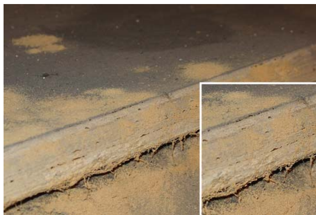
Fig. 2 Coffin lid showing fresh bore dust, tunnelling by the larvae, and feeding striations on the wood surface by adult P. huttoni (inset: detail view)
